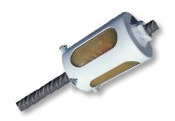
The RBM-VX<sup>TM</sup> is an Industrial Internet of Things (IIoT) device for real-time rock bolt monitoring to ensure the stability of mines and safeguard lives. It is designed to support resin installation and pre-tensioning using jumbos with no, or minimal, human interaction.
